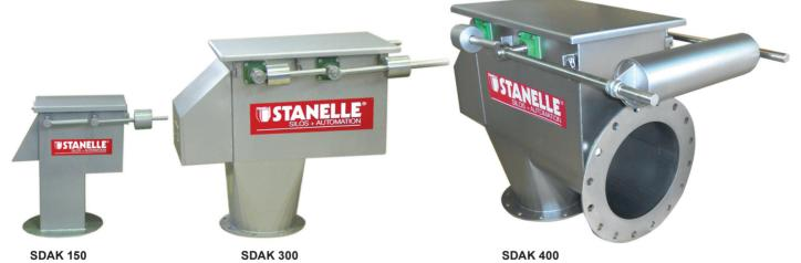
Areas of application: The Stanelle-Overpressure and Vacuum Flap, Type SDAK, is a safety organ for silos which are filled pneumatically. Overpressure as well as vacuum – the latter arising from exhaust fans or through cornice collapses – can be balanced because of the combined design of the pressure flaps. The optimum protection of the silo is guaranteed through the maintenance-free construction of the SDAK flaps.
